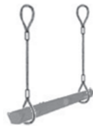
"Bilancino" (1 truss beam + 2 suspension points)
